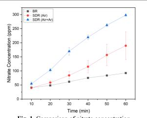
**Fig. 1**. Comparison of nitrate concentration evolution in the bubbling reactor (BR) and spinning disc reactor (SDR).
